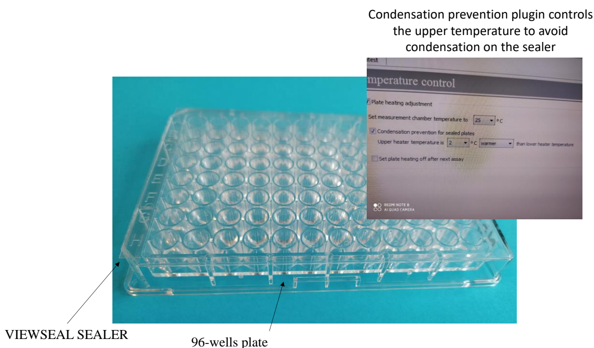
Figure S 9. 96-wells plate, sealer and condensation prevention controller from ENVISION multimode microplates reader (Perkin Elmer) used for kinetic measurements.
